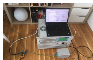
Measurement of grid impedance at an outlet
