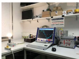
Laboratory measurement of heating due to supraharmonics
