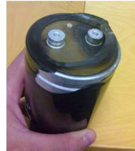
Destroyed DC-link capacitor of a UPS
